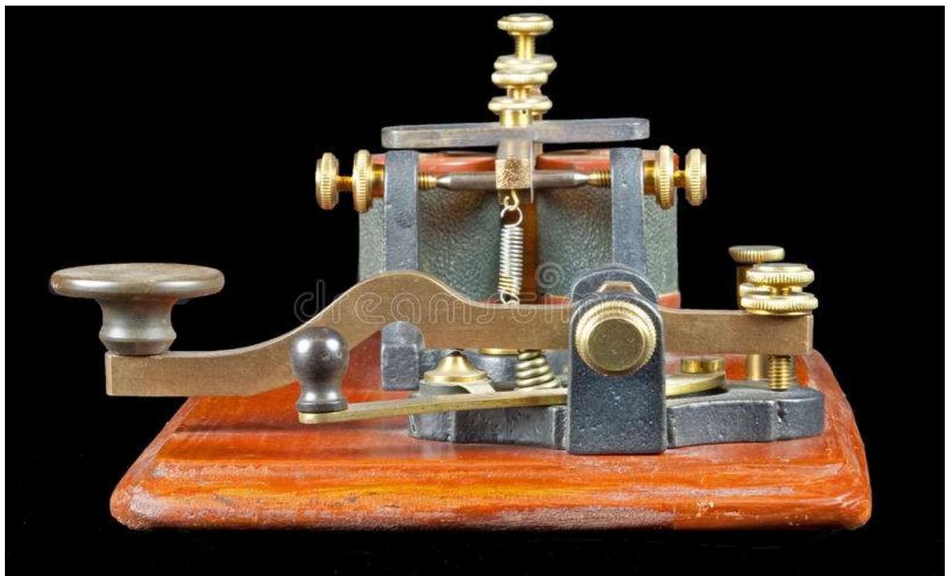
Portable Camelback key and sounder on wood from mid-19 th century. These were sometimes used to link army units in pitched battle situations by generals like William Tecumseh Sherman in the American Civil War.
